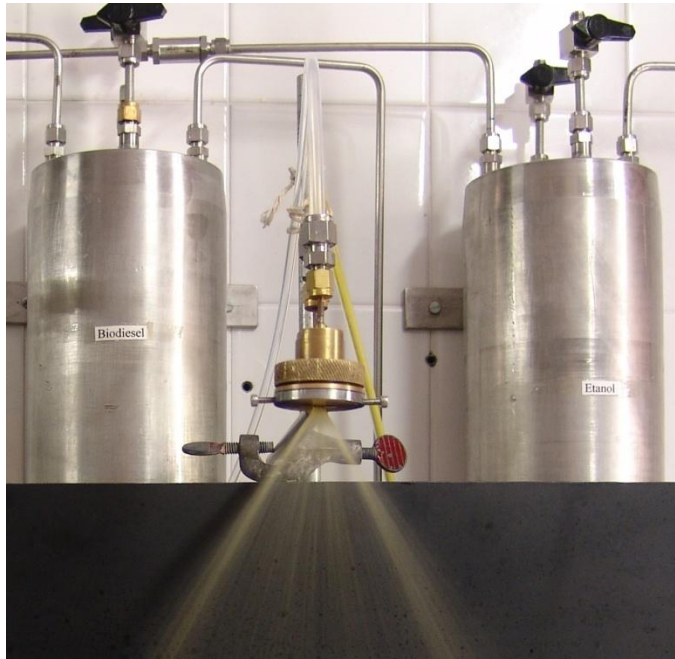
Spray of the ethanol and biodiesel mixture with 1 bar manometric pressure.
