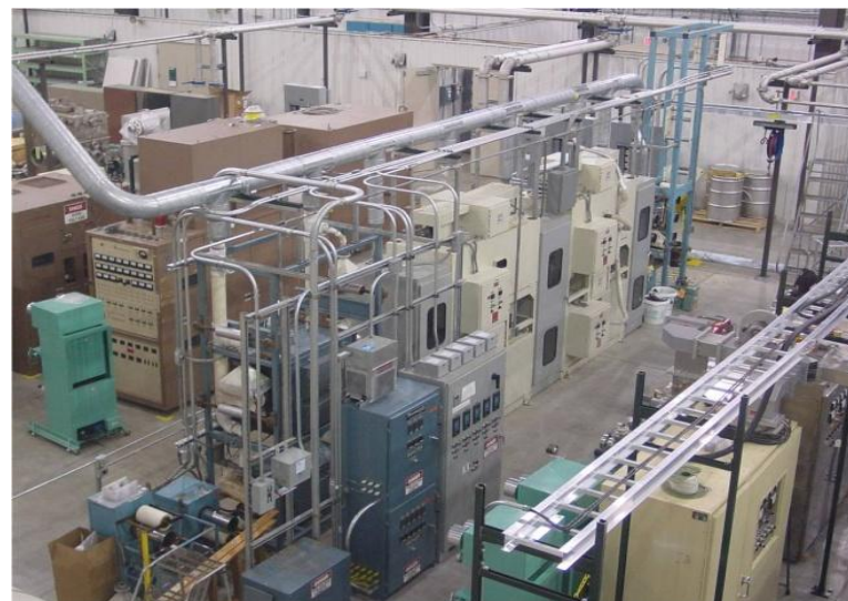
Pilot-scale, multiple-tow carbon fiber conversion line ( \approx 20 lb/day)
