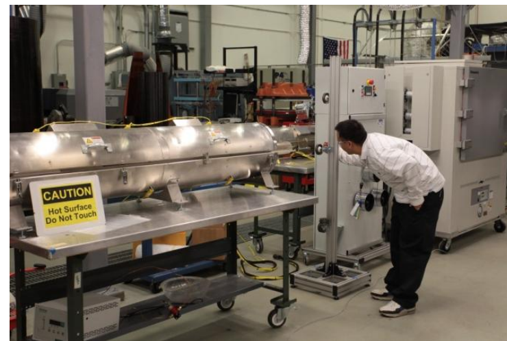
Oxidized fiber entering carbonization furnace
